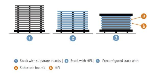
If the composite element (HPL and substrates) to be fabricated will be constantly exposed to low relative humidity during future use, it is recommended that the HPL and substrate be exposed to the corresponding humidity during conditioning to estimate the shrinkage stress that occurs subsequently.
